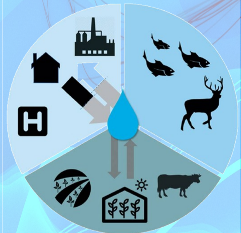
The water system as integrator of urban and rural water withdrawals and returns, where sectors and nature demand sufficient water quality fit for purpose. Arrow widths summarize volumes abstracted in the EU context (FAO AQUASTAT data) for urban withdrawals (industry and municipalities) and rural withdrawals (agriculture); arrow darkness represents the presence and concentration of chemicals.
